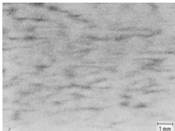
Figure 1 Low magnification micrograph of heat treatment 6R showing overview of carbon segregation.
